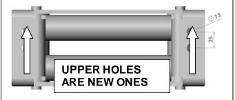
51. If necessary, mark out and drill two new 13mm holes in the roller fairlead, 25mm apart from the original holes, as shown on the adjacent picture.
