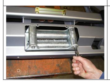
52. Place roller fairlead over lower holes and again secure using 3/8" hardware (1 3/4"x 3/8" bolts) flat and spring washers.
