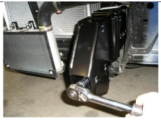
26. Fit impact absorbers as shown using existing horizontal and vertical bolts from crash bar first applying loctite thread locker, as in steps 21 &22. LHS shown (note the RHS and LHS orientation)
