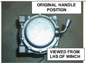
46. To fit an 8/9/9500lb winch, you will need to rotate gearbox 144° (4 x hole spaces) counter clockwise.
