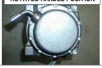
47. Stand winch upright and undo the cap screws and by lifting the gearbox only a couple of millimeters, rotate the gearbox.
