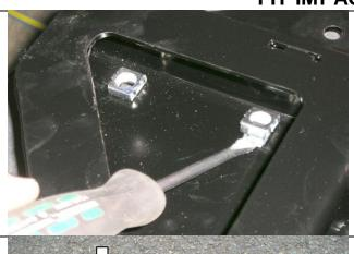
24. Fit M10 cage nuts to impact absorbers as shown, use a screwdriver to assist pushing in flange.
