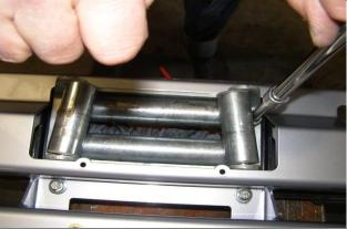
54. If circlips were removed, refit rollers and circlips after tightening bolts.
