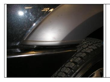
75. Clean surface of flare and fit rubber edging as shown.
