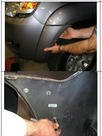
10. Pull outer wings of bumper as shown, when both sides are released carefully remove bumper and place on soft surface to prevent damage.
