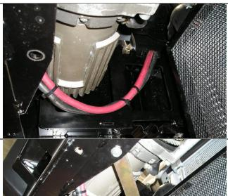
67. When bar is secured to mounting bracket, connect winch cables to battery and cable tie cables together clear of all moving parts, sharp edges and hot parts.
