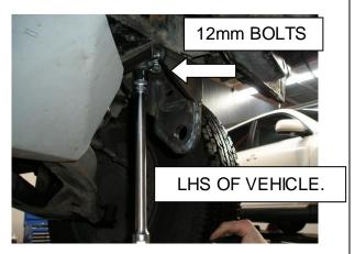
31. After fitting impact absorbers to vehicle, the brace assembly is next to be fitted.
