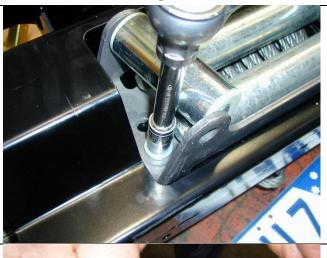
53. Tighten all bolts using socket and extension.
