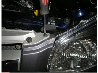
6. Remove screws holding grille in place
