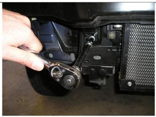
23. Undo horizontal bolts and remove crash bar from vehicle and set aside. Retain the 4 x bolts for reuse.
