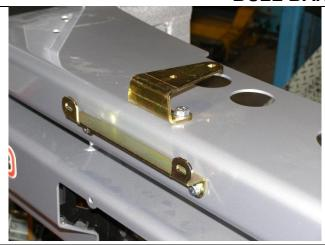
If you are not going to fit a winch to the bar, go to step 64. Non winch application number plate fitment is at step 86
