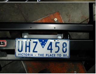
78. If the bar is a non winch bar setup, the number plate is fitted to front of bull bar directly as per photo using press in 2 x large round head plastic grommets and black Philips drive pan head screws. This position will cover the roller fairlead cutout in pan.
