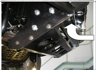
73. Fit M6 caged nuts to air deflector and fit in between lower section of bar and secure using M6 hardware.
