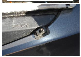
69. Fit light insert into bar. Secure using 4 screws, rubber washers and retainer clips from inside rear. (Do not over tighten)
